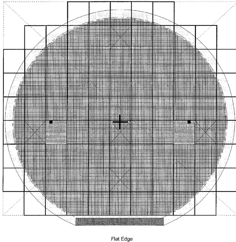
Die:  $0.894 \times 0.864$ , Step:  $0.994 \times 0.934$ , N:  $14 \times 7$ , Frame Step:  $13.916 \times 15.878$
