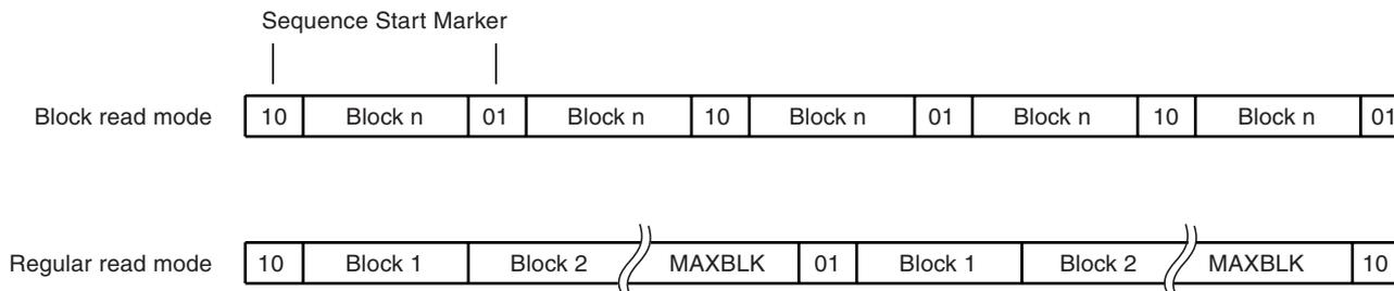
The ATA5567 sequence start marker is a special damping pattern, which may be used to synchronize the reader. The sequence start marker consists of two bits (“01” or “10”) which are inserted as a header before the first block to be transmitted if bit 29 in extended mode is set. At the start of a new block sequence, the value of the two bits is inverted.
