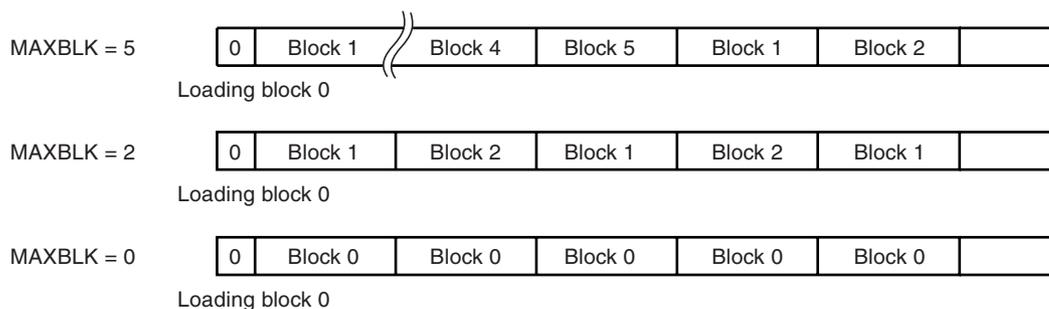
Every time the ATA5567 enters regular-read or block-read mode, the first bit transmitted is a logical 0. The data stream starts with block 1, bit 1, continues through MAXBLK, bit 32, and cycles continuously if in regular-read mode.
