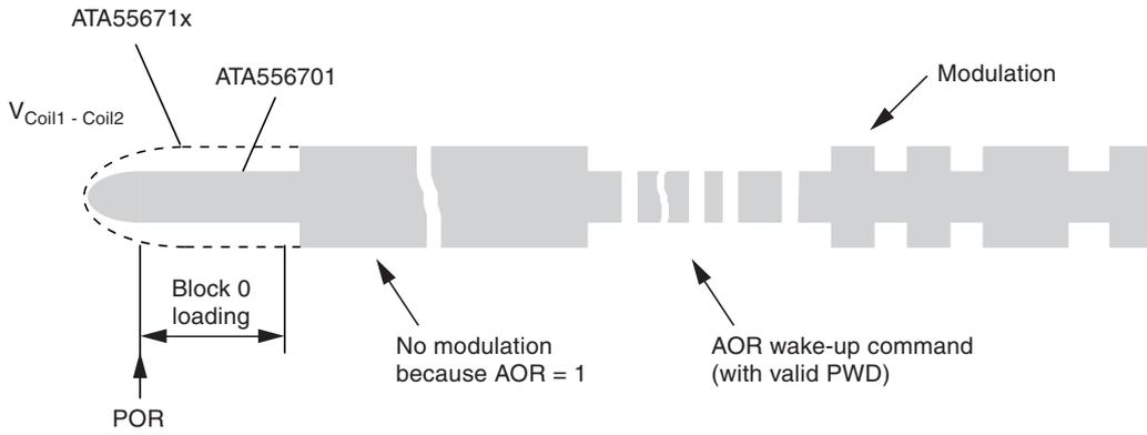
**Figure 4-8.** Coil Voltage after Programming of a Memory Block
