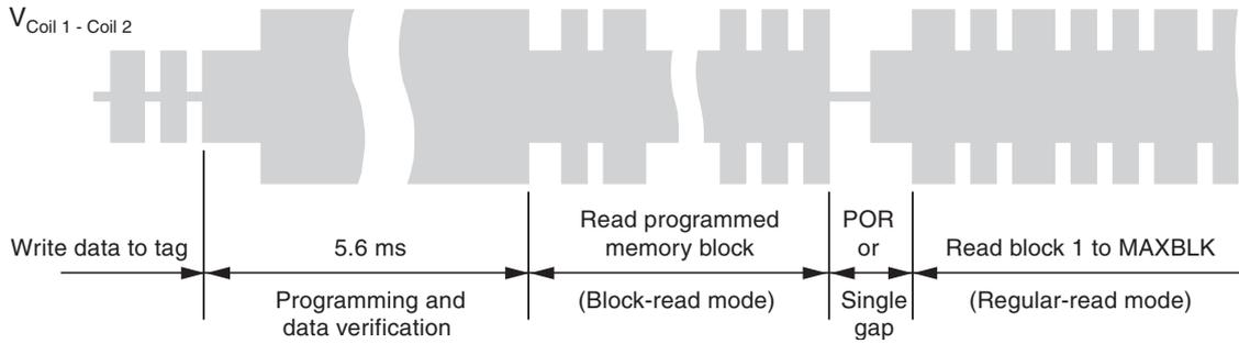
Figure 4-9. Anticollision Procedure Using AOR Mode
